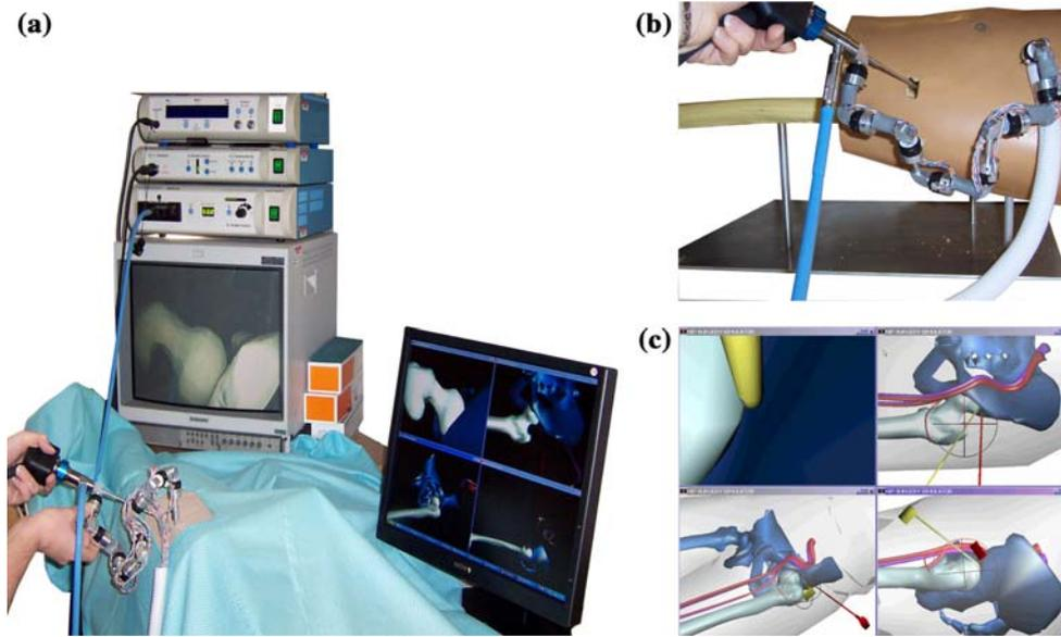
**Fig. 1** Computer-aided arthroscopic hip surgery system from [8]. **a** Setup of complete computer-aided system with Smith and Nephew arthroscopic equipment [9]. **b** Encoder linkage tracks an arthroscopic
