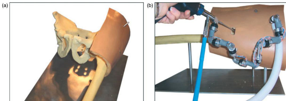
Figure 9. Hip model and arthroscope connections. (a) Model of human hip joint. (b) Arthroscope and linkage applied to model. The arthroscope must be connected to both the tracking chain and traditional arthroscopic equipment (camera head and light source)
