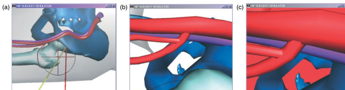
Figure 8. Proximity warning system. (a) Sphere representing safe area for tool operation. (b) Arthroscopic view from within the safe sphere. (c) Arthroscopic view from outside the safe sphere. As the arthroscope moves outside of the spherically-defined safe region and toward the femoral artery, the screen background changes to red to warn the surgeon
