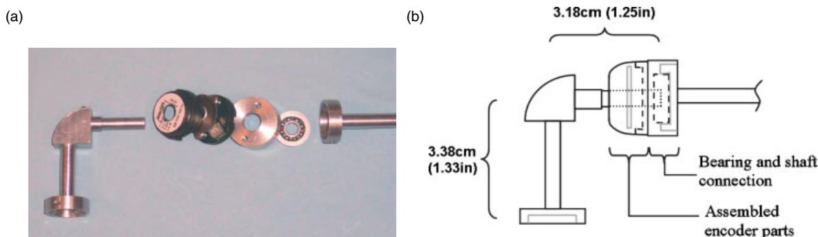
Figure 4. Encoder link components (a) and assembly. (b) Diagram of the assembled link
