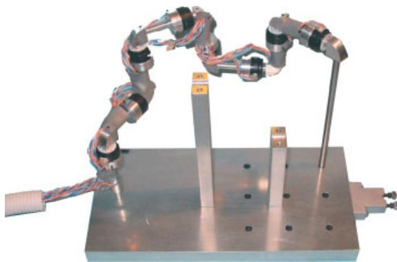
Figure 11. Encoder linkage with generic tool inserted in one of machined holes
