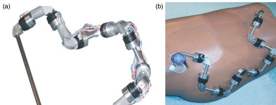
Figure 3. Encoder linkage for position tracking. (a) Tracking linkage prototype. (b) Linkage applied to a hip model. The linkage is redundant with extra degrees of freedom, to increase flexibility and ensure that the linkage remains out of the surgeon’s work space
