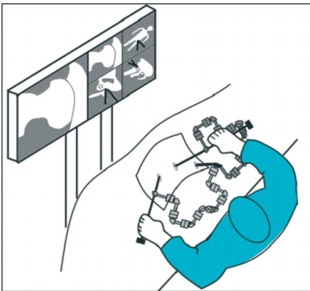
**Figure 2.** A computer-aided navigation system for arthroscopic hip surgery using a linkage tracking mechanism. Two encoder chains track the position of the surgeon's arthroscope and other tools. An additional screen in the operating room displays computer images of instruments and the patient anatomy from multiple views
