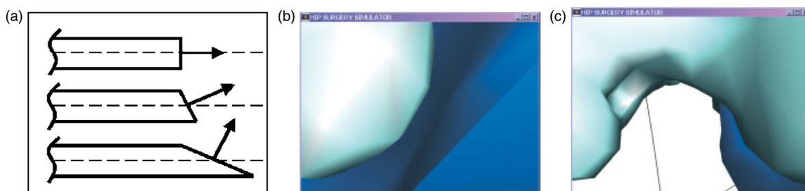
Figure 7. Comparison of arthroscopes with varying viewing angles. The camera angle describes the camera viewing direction; the angle is measured from the axial direction of the tool to the viewing direction. (a) Arthroscopes with 0° (top), 30° (centre) and 70° (bottom) viewing angles. (b) Computer-generated view from arthroscope with 0° viewing angle. (c) Computer-generated view from arthroscope with 70° viewing angle
